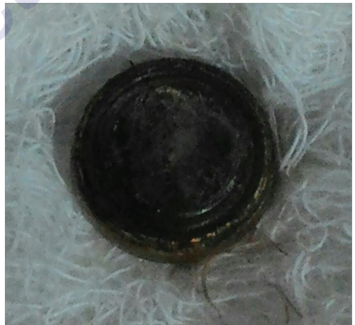
FIG. 2. Picture of the leaked button battery.
