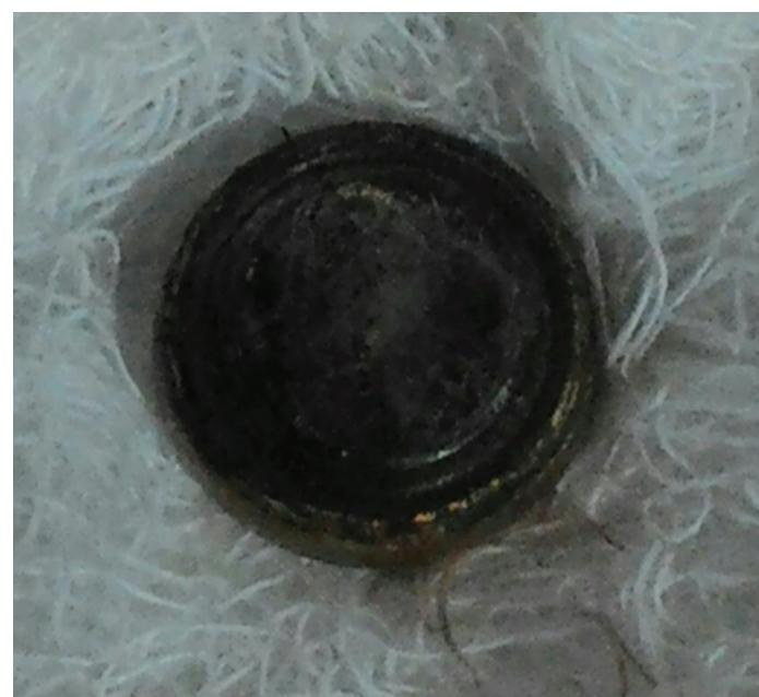
**FIG. 2.** Picture of the leaked button battery.
