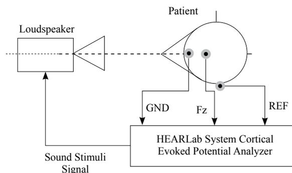
**FIG. 1.** The CAEP measurement setup
