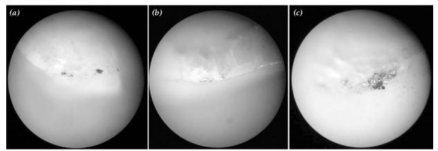
Fig. 3. (a) (+) Metallic residue; (b) (++) metallic residue; (c) (+++) metallic residue.
