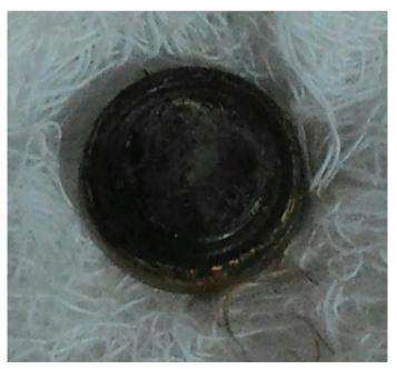
FIG. 2. Picture of the leaked button battery.
